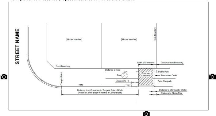
Photos of existing infrastructure should be taken from the 3 points as indicated above. The photos should capture all of the infrastructure indicated within the drawing.
