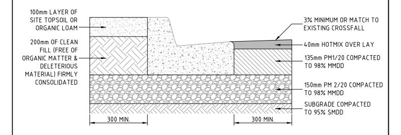
150mm BARRIER KERB AND GUTTER REINSTATEMENT SCALE 1:10
