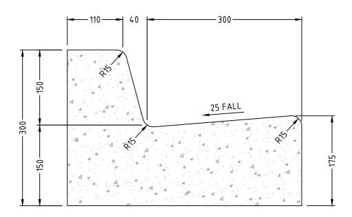
150mm BARRIER KERB AND GUTTER
