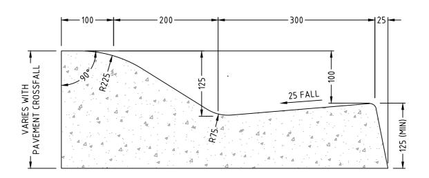
SEMI MOUNTABLE KERB AND GUTTER
