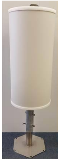
Figure 5: The pod solution (concept under trial) includes antennas/radio units all in one unit.
