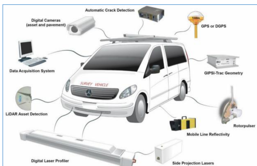
High Speed Data Vehicle – Provides detailed information about the seal condition
