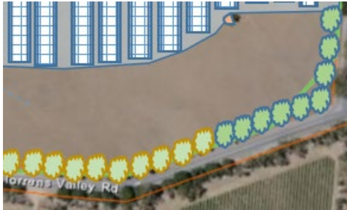
Fig.3. Inset showing location of vegetation buffer along Torrens Valley Way and the section of Warren Road currently not fully screened. The width of the vegetation buffer will be 3m.
