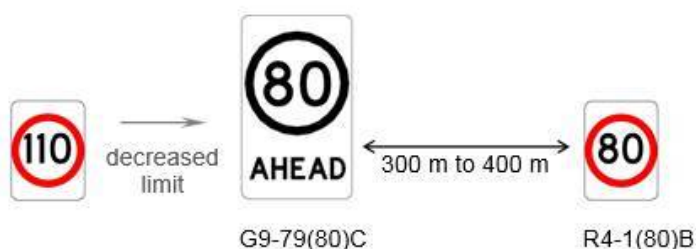
Figure 3.31 Reduction from 110 km/h to 80 km/h
