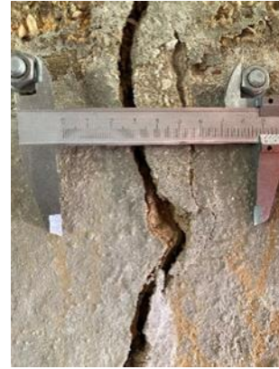
Figure 2.26 Installed anchorage bolts spacing, left-hand side of abutment 2 – 90 mm
