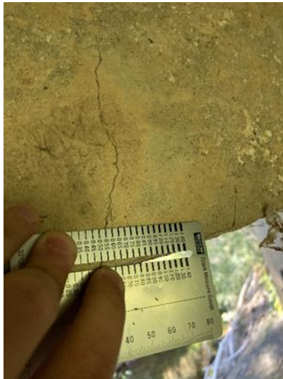
Figure 2.6 Moderate flexural crack, 0.55 mm wide and located at mid-span of girder 2
