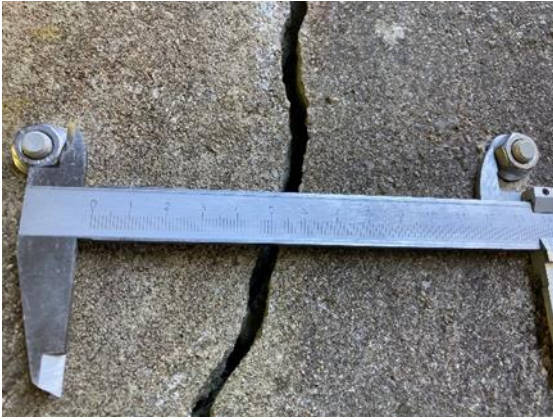
Figure 2.12 Bolts spacing recorded as 125 mm
