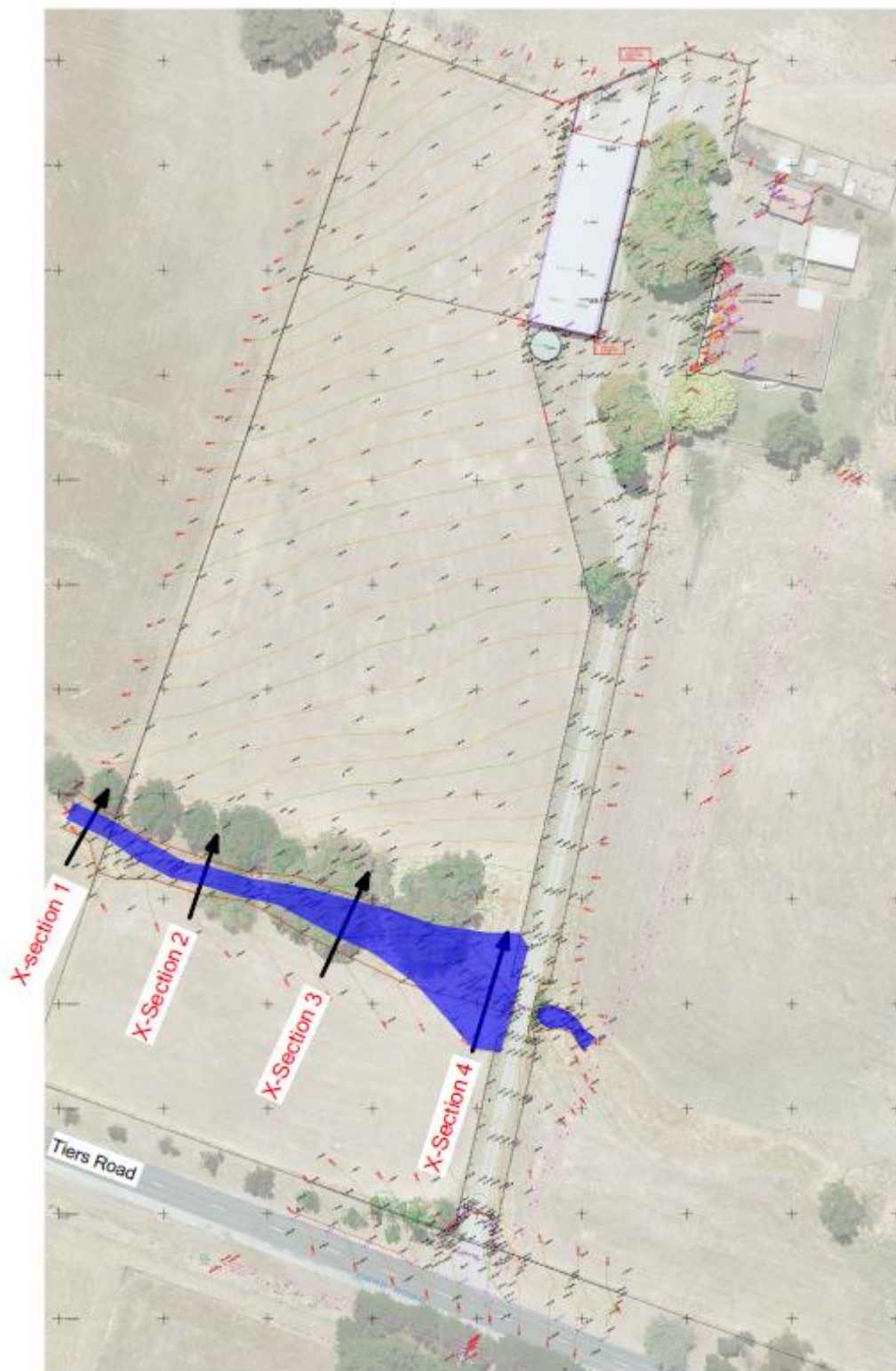
12 Tiers Road, Woodside Watercourse Cross-Section Location and 10% AEP Flow Surface Plan
