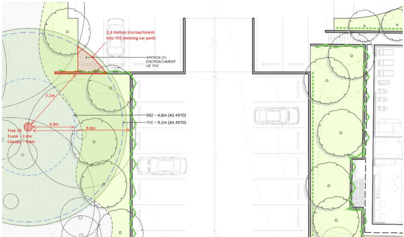
Figure 1 – Mark-up diagram (Landskap base plan) identifying AS 4970 TPZ and SRZ and extent of encroachment of existing car park surface.
