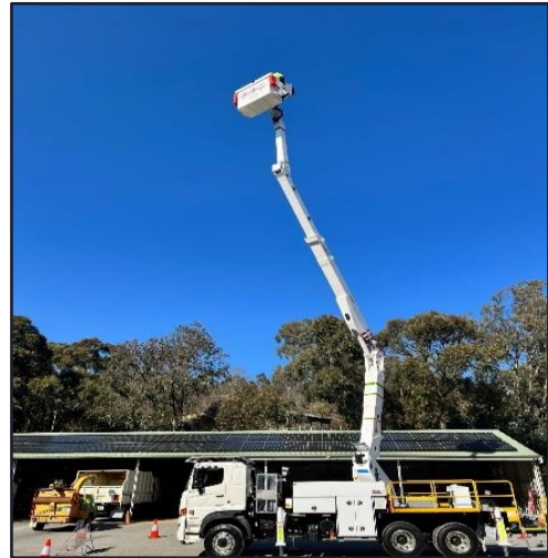
Shows the maximum height of the EWP which is 19m.
